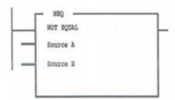
Use the NEQ instruction to test whether two values are not equal. If source A and source B are not equal, the instruction is logically true.
