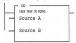
Use the LEQ instruction to test whether one value (source A) is less than or equal to another (source B). If the value at source A is less than or equal to the value at source B, the instruction is logically true.
