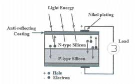
These electrodes do not obstruct light to reach the thin p-type layer. Just below the n-type layer there is a p-n junction. We also provide a current collecting electrode at the bottom of the p-type layer. We encapsulate the entire assembly by thin glass to protect the **solar cell** from any mechanical shock.
