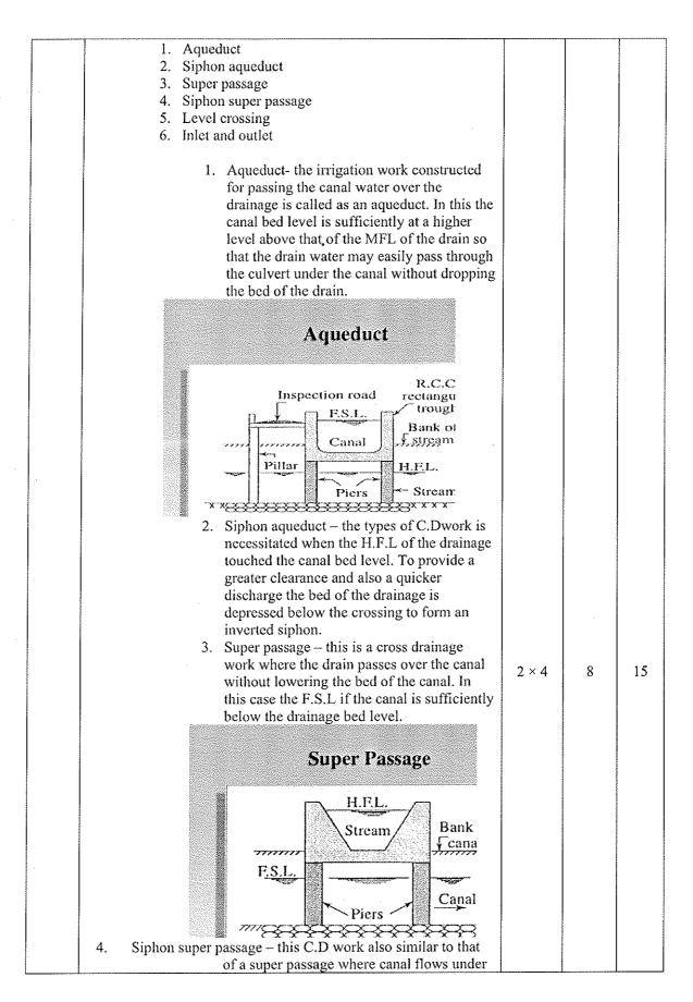
the drain. If the F.S.L of the canal is not sufficiently below the bed level of drainage, the water of canal is to be siphoned through the drain by lowering the bed of the canal.
